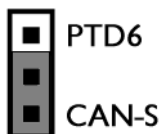
Figure 8-4: Can Operation Mode Selection (J6)
